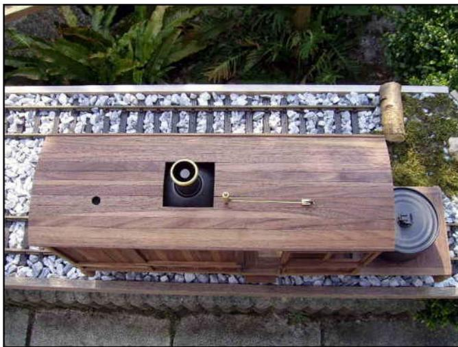
The hole in the roof is for filling/accessibility gas tank.
