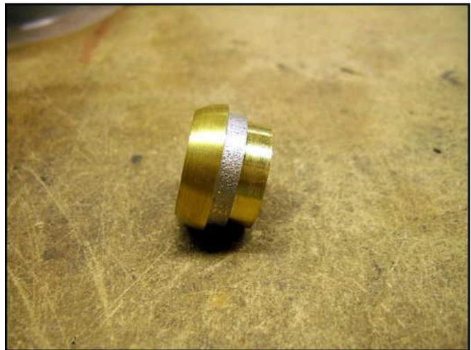
I've created an adapter - burner is 18 mm - pipe inside diameter 19 mm.
