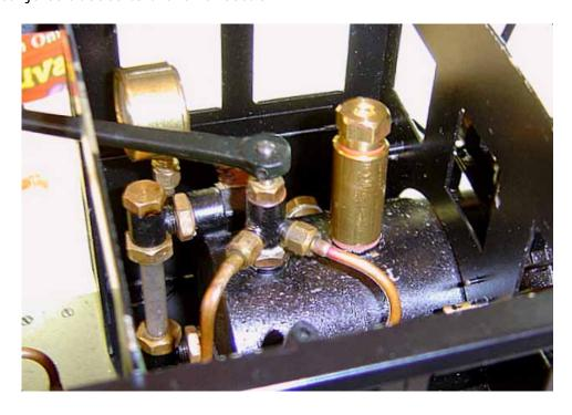
Here's the original Goodall Valve. Great for the boiler refilling function it is made for, but we'll be scrapping the main body and turning up a new piece which incorporates the banjo bolt
