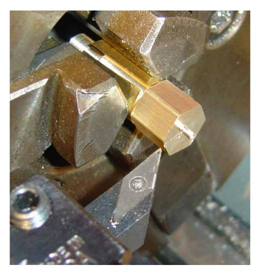
Here's the finished banjo bolt showing the Goodall valve and also the banjo fitting with steam tube. The banjo fitting "donut" is a simple straight turned piece with a bore just large enough to slide over the shoulder on the banjo bolt. This shoulder is seen just above the cross drilled hole in the turned down area of the banjo bolt. In use the bolt tighens down on the banjo fitting donut and with the red fiber washers shown creates a steam tight seal.
