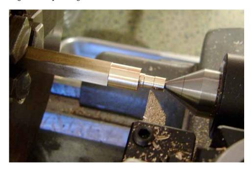
Now we come to drilling the hole through the Banjo bolt. Normally this hole would only extend up to the turned down area with the upper portion of the bolt remaining solid. In this application, however, I wanted to keep the Goodall valve function so the bore extends clear though the bolt and we will later add treads to the top for the Goodall valve to screw into:
