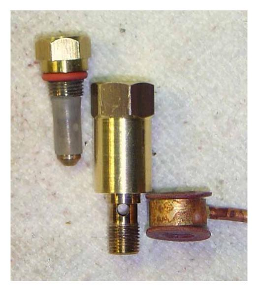
And here's two views of the new banjo bolt and fitting in use with the whistle installed and functioning. Using the custom made banjo bolt and fitting retains use of the Goodall valve, and makes for a neat and tidy installation:
