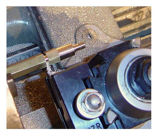
Now that the banjo bolt has been cut off, it is turned around in the lathe chuck, and in this photo is being faced off in preparation for boring and internal threading. This is the top of the banjo bolt where the Goodall valve will screw into. Note also that small pieces of shim stock are being used on the jaws of the lathe chuck to protect the finished outer surface of the banjo bolt:
