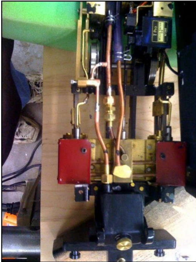
Finished lubricator mounted with adjustment valve on the left.
