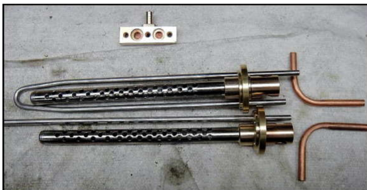
Burners with front and rear super-heaters, steam manifold and connection tubes. Note "U" shaped super-heater, which goes back to the rear engine.
