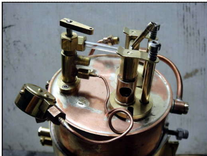
Boiler backhead showing throttle valve, sight glass, pressure gauge and spring held jets.
