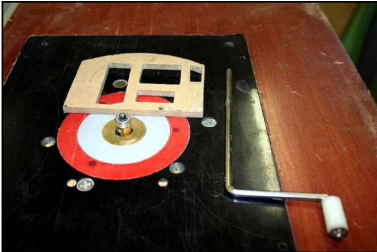
Router with pattern making setup, note the almost zero clearance between the table opening and the cutting tool.
