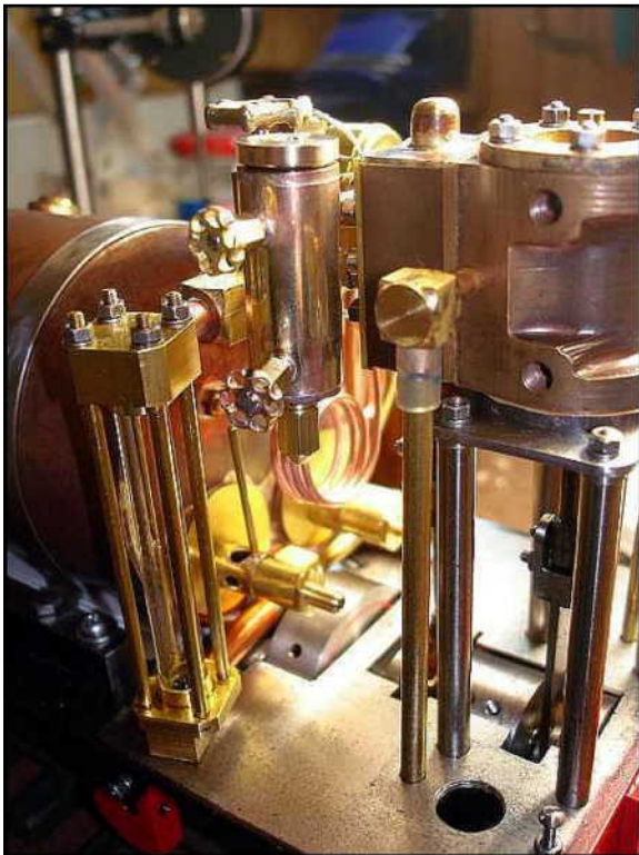
Lubricator with new steam feed valve at the bottom.
