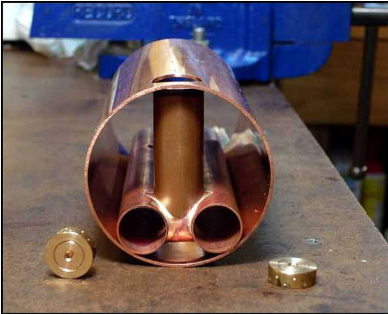
Boiler internal assembly.
