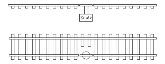
Basically a section of rail long enough for one wheel is removed from a section of track and attached to a scale such that it is even in height with the rails sections on both sides. The loco is then positioned on the track such that each driver is weighed in turn. Face the loco the other way and weight the other side.
