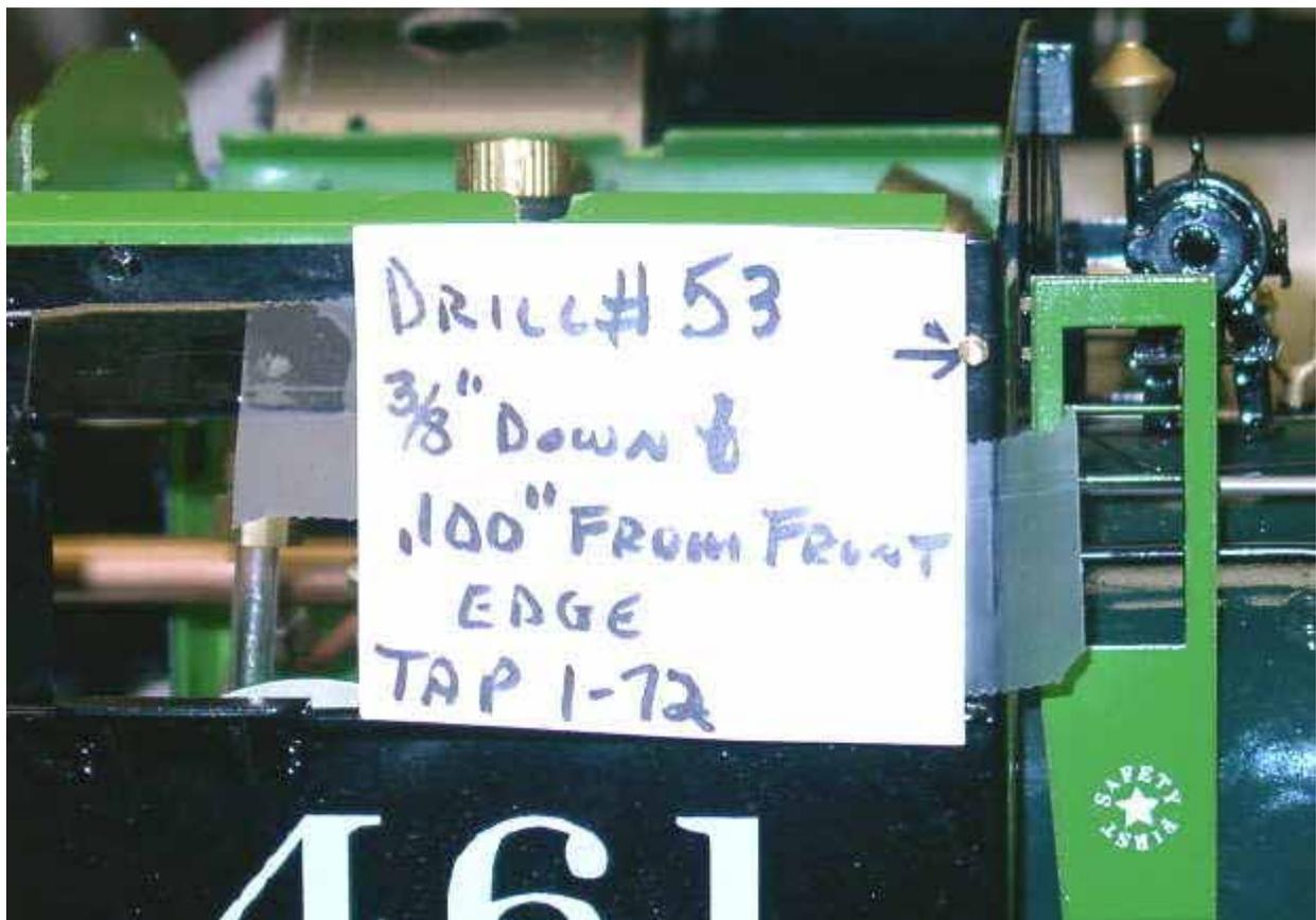
Back one of the 1-72 bolts out & install that hinge assembly you made a while back. All that holds it in is those two bolts.
