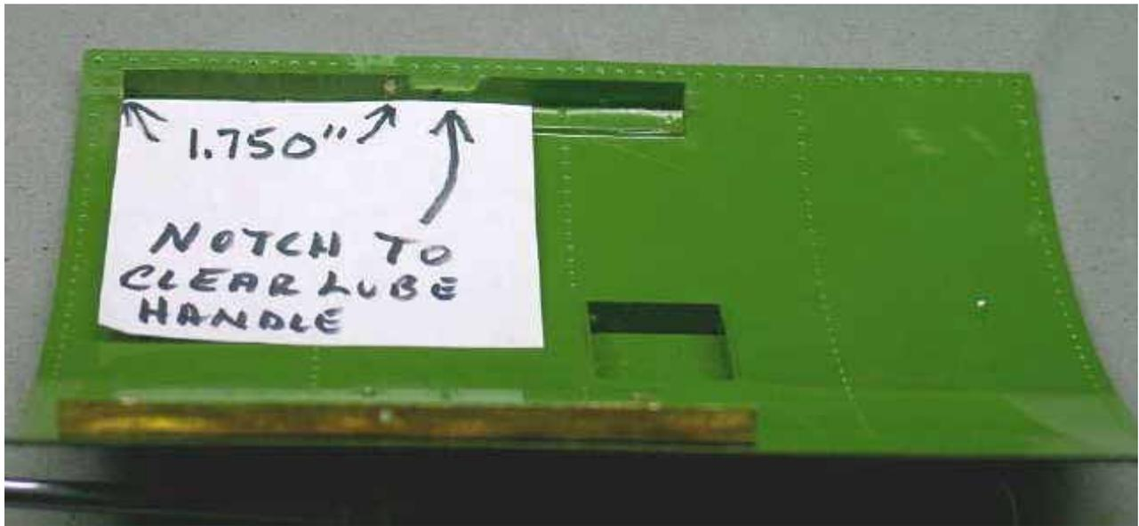
Drill & tap the cab front side plate as shown. Drill #53 hole, 3/8" down from the top edge of the side panel and .100" in from the front edge. Tap this 1-72. A 1-72 model bolt or screw 1/4" long goes here as the hinge pin.
