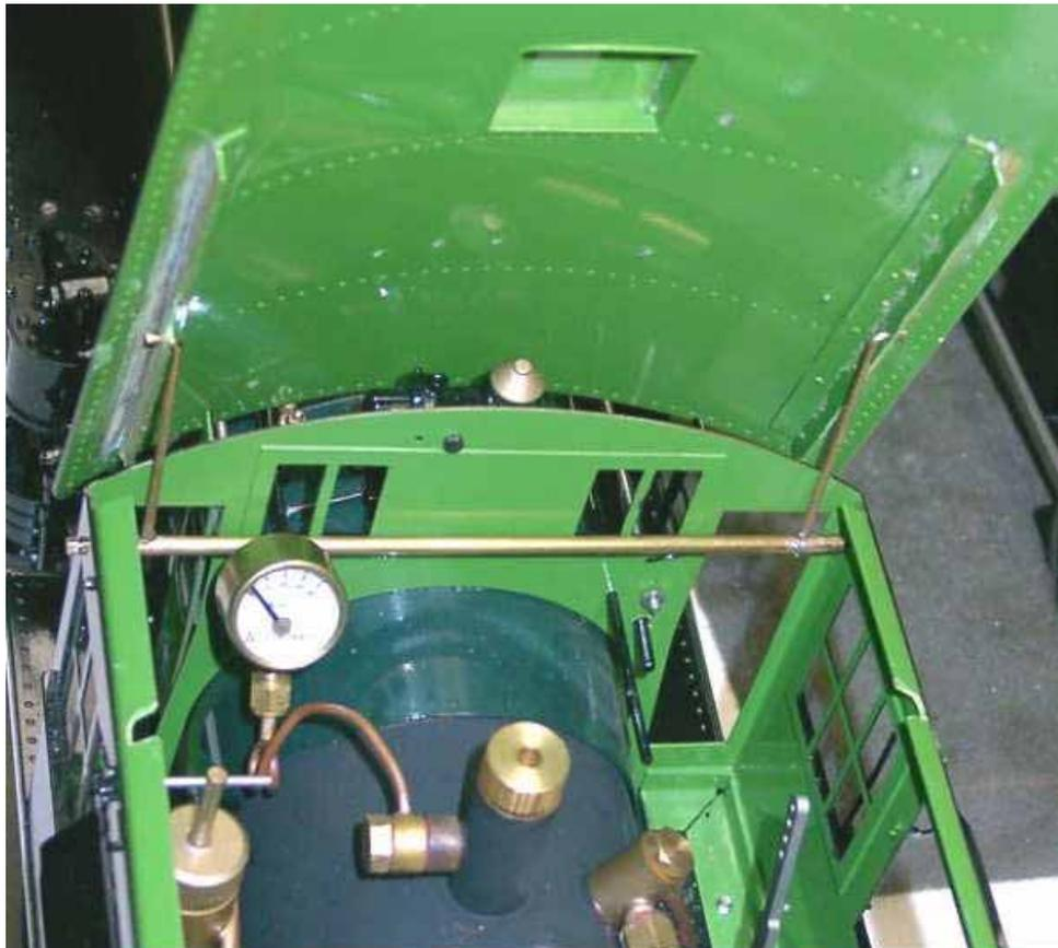
To check pressure or adjust the throttle all you have to do is stick your hand or pinkey in and lift the roof. Now is probably also a good time to do some painting & touchup so the parts won't be so noticeable. The parts on mine are now painted flat black and the 2 bolts on the cab sides are gloss black. That's my first run shown below coming out of the Square Roundhouse.
