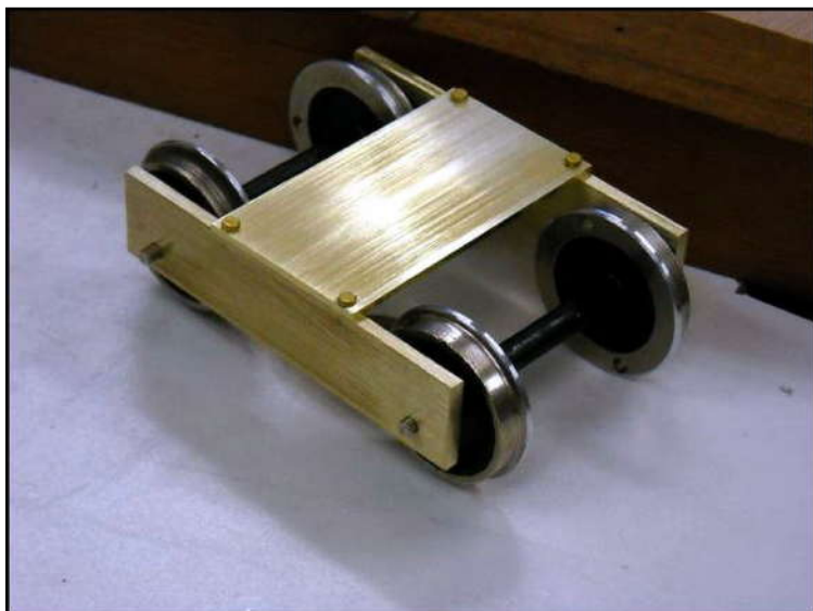
The wheels are some old Bachman ones I had laying around. I turned the flanges down on the lathe. The sides are 1/8" bar stock and the top 1/16".
