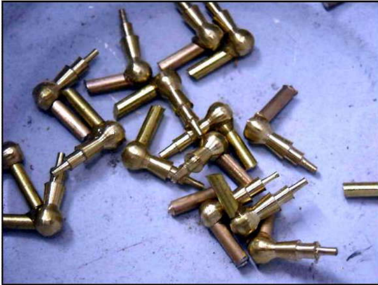
Door handles turned on the lathe. Ends were rounded over on the grinder
