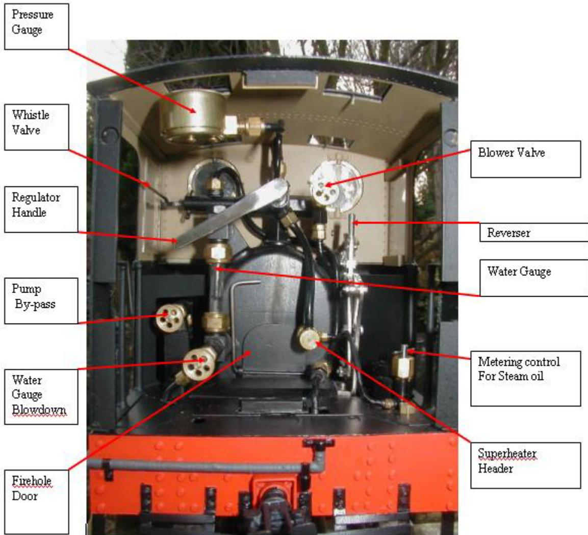
**Cab Controls on Coal Fired L&B LEW by DJB Engineering**
