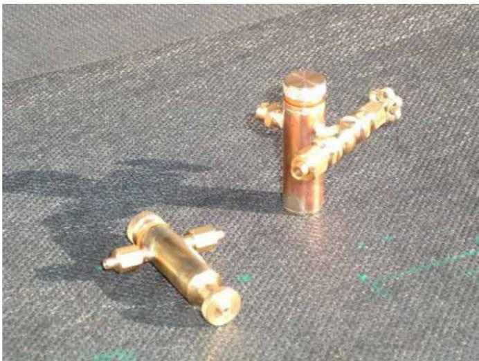
I assumed these acted as I believed all did, the needle valve provides metering control of the amount of oil that combines with the Steam. But the reply I received from ACS below describes two of their lubricators as actually steam throttles, metering the amount of steam to the cylinders with a constant volume of steam oil added to the steam. Their lubricator body is 2" x 5/8" dia, add 1/2" for either the drain or vertical control wheel, with both the total height is 3":
