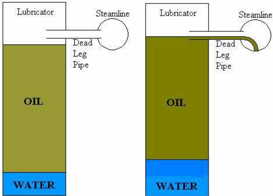
This is a cross section of a lubricator attached to the steam pipe by a short leg of smaller tubing, ie, a "dead leg connection." In fact this leg of tubing can be so short that it is nothing more than the hole in the steam pipe as the steam pipe passes through the lubricator, a "pass through connection." The lubricator is closed on the top, unlike the glass of water it has no brim, but it does have a hole in its side, the tube leg.
