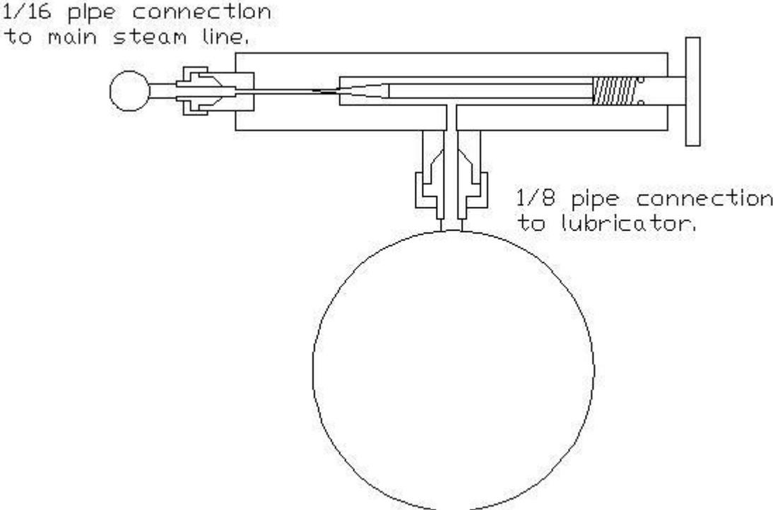
Needle Valve through the center of lubricator:
