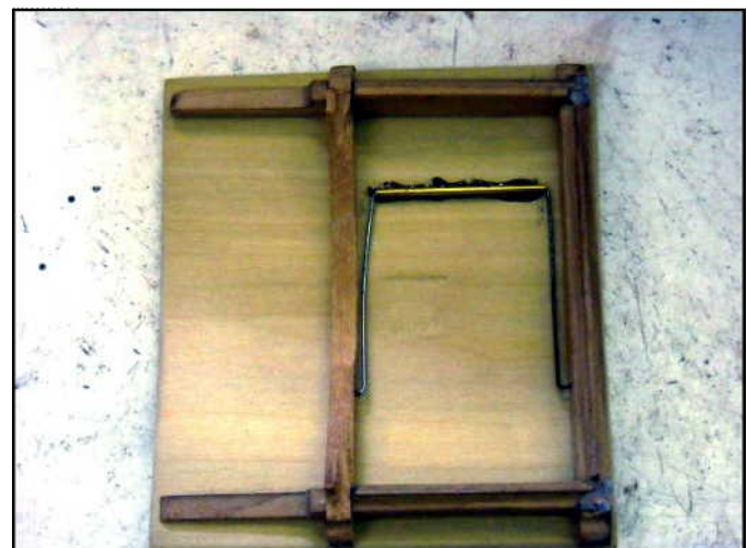
Hinge for roof is attached with JB Weld.
