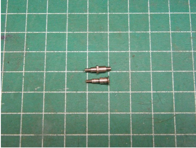
New cross head pin above the OEM pin
