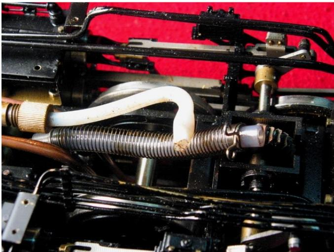
THE COMPLETED MECHANICAL PIVOT (HEREINAFTER KNOWN AS A DOG BONE) IS COMBINED WITH AN OIL LINE SEPARATED FROM THE SUPERHEATER TO AVOID COKING OF THE OIL AND PREMATURE FAILURE OF THE DOG BONE O-RINGS.
